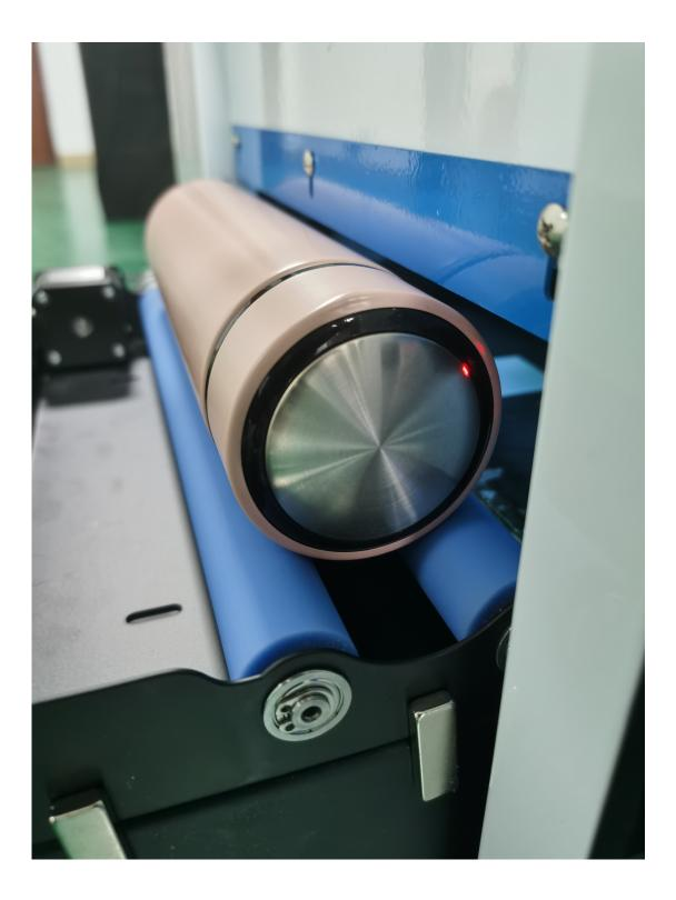
**3**.Disconnect the cable and connect it to the cylindrical fixture.
