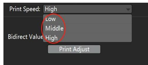
Finally, switch to different speeds to calibrate the two-way printing values and save them separately.
