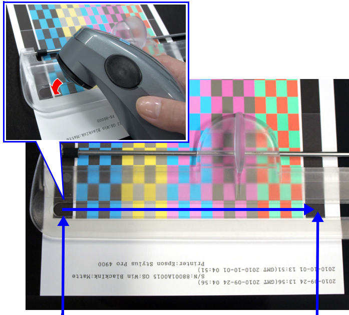
Figure 5-97. Setting the Calibrator/Measuring Position
