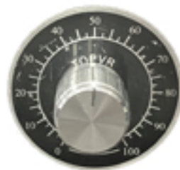
White ink circulating pump power adjustment knob
