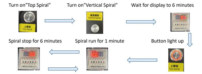
The spiral runs for 1 minute, stops for 6 minutes, continues to run for 1 minute, stops for 6 minutes, and repeats continuously.
