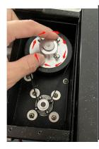
After the accessories installed, are manually rotate the screw clockwise to check whether the rotation is smooth and whether there is any abnormal noise.
