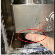
After the manual rotation is confirmed to be smooth, do not add powder first, turn on the power and start the spiral rotation. Let the screw rotate for about 30 minutes without load, and gently touch the stainless steel outer wall with your hand to check whether it is hot. If there is a hot hand (over 55  $^{\circ}$  C), it is abnormal, and the installation needs to be re-checked.
