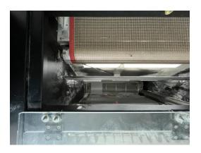
2 Bracket fixed Remove the two screws marked in the picture, fix the bracket, and fix the bracket with two screws longer than the original.
