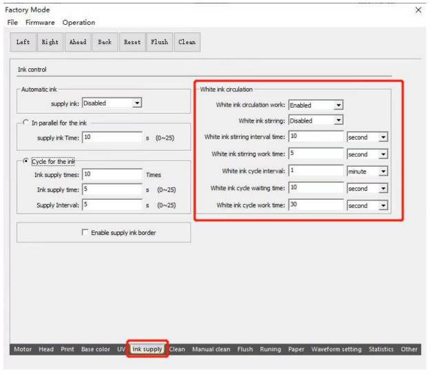
White ink circulation work: Enable/Disable (Enable: Pump work timing, Disable: Pump stop)
