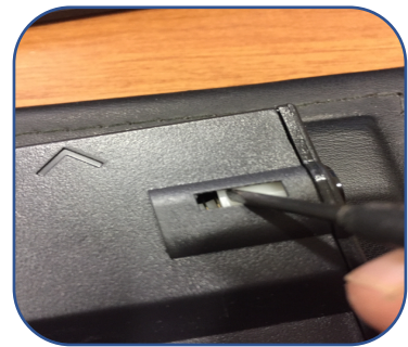
Paper Tray spring lock disengaged
