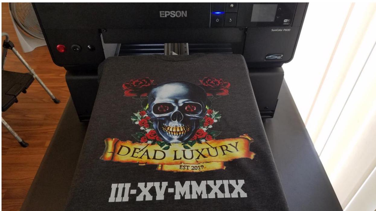
"In the RIP software, I switched the underlying layer to *100% white* and the *output to 80%* (because the white wasn't as vibrant at first). Then on the second pass I switched it back to *white gradient underlay*. Then ran the color print on top. A double pass worked."
