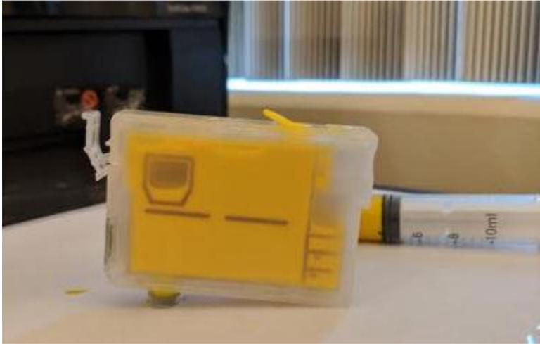
Ensure the clear plastic plug is removed allowing the air vent hole to be open.
