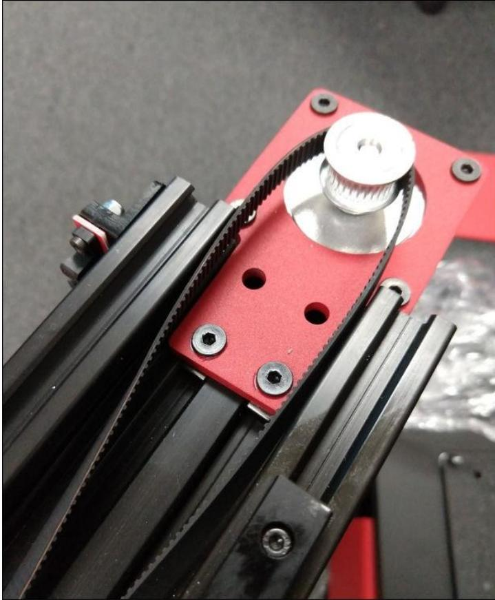
You may notice oil on the rail edge. Do not wipe, this is lubrication for the moving of the track arm on the rail.
