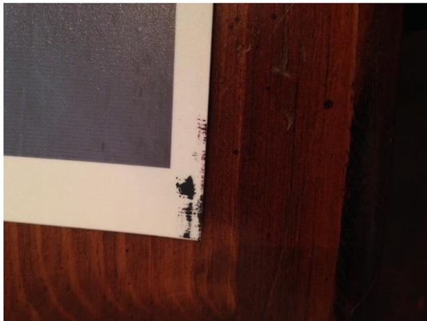
Optimal DTG printing is done with the fabric at 2-3mm below the Printhead. Note that, Prints will appear BLURRY and with ink spray edges, if the correct distance is not achieved.
