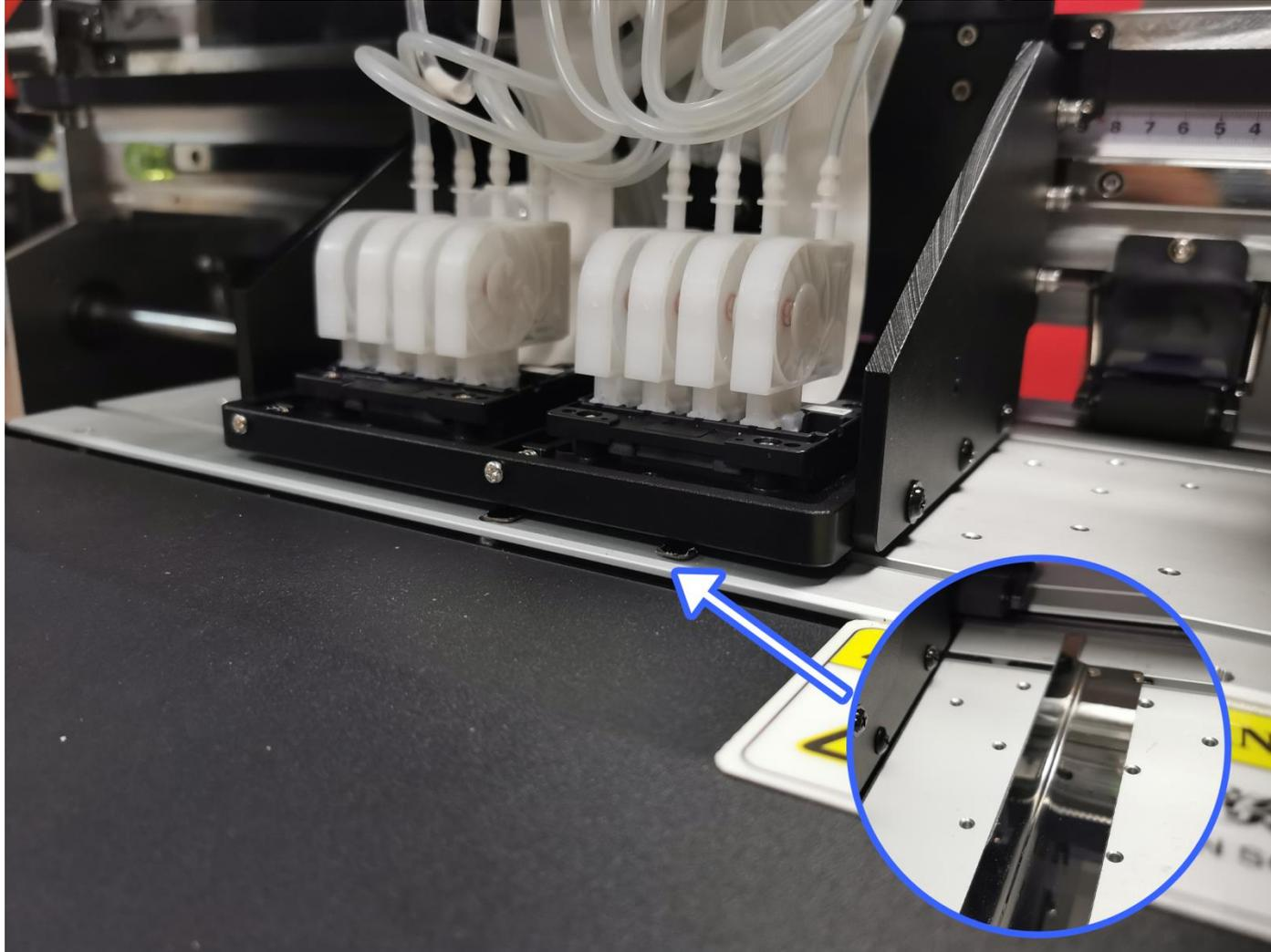
1. After installing the print heads and ink dampers, please move the print head bracket slowly to check whether the print head will scratch the paper pressing sheet
