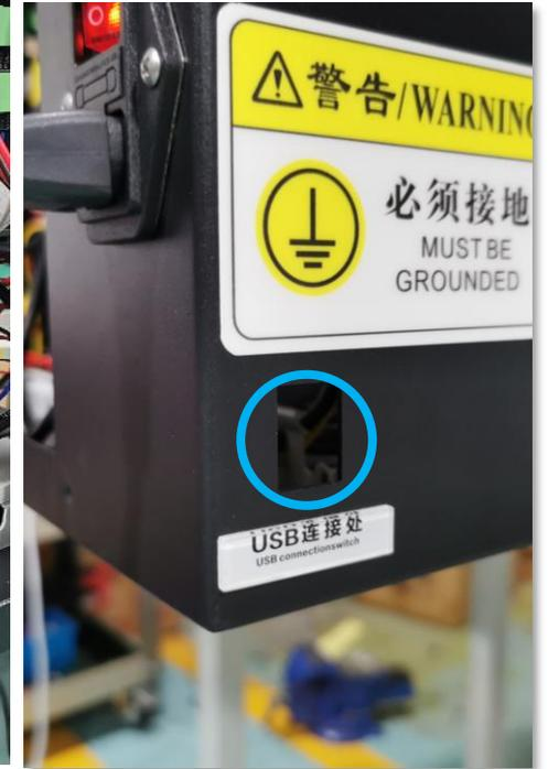
Pass the blue circle marked network cable through any hole and connect it to the computer
