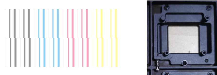
3. Until the nozzle prints the following picture vertically, this state means that the nozzle has been vertical.
