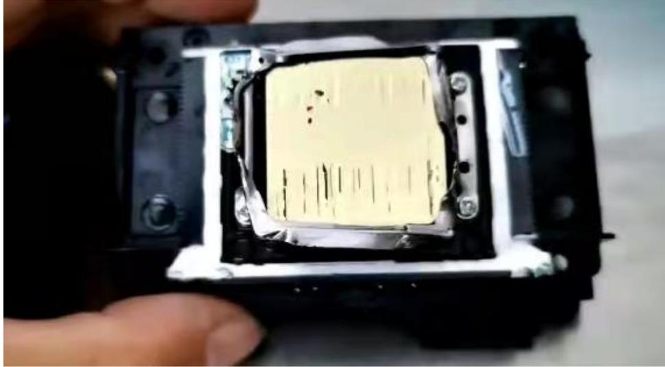
The Nozzle cannot be used after being scratched
