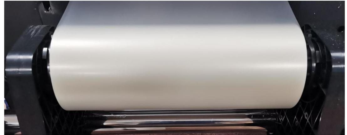
2. Pull down the handle, and the paper pressing roller will lift up at the same time
