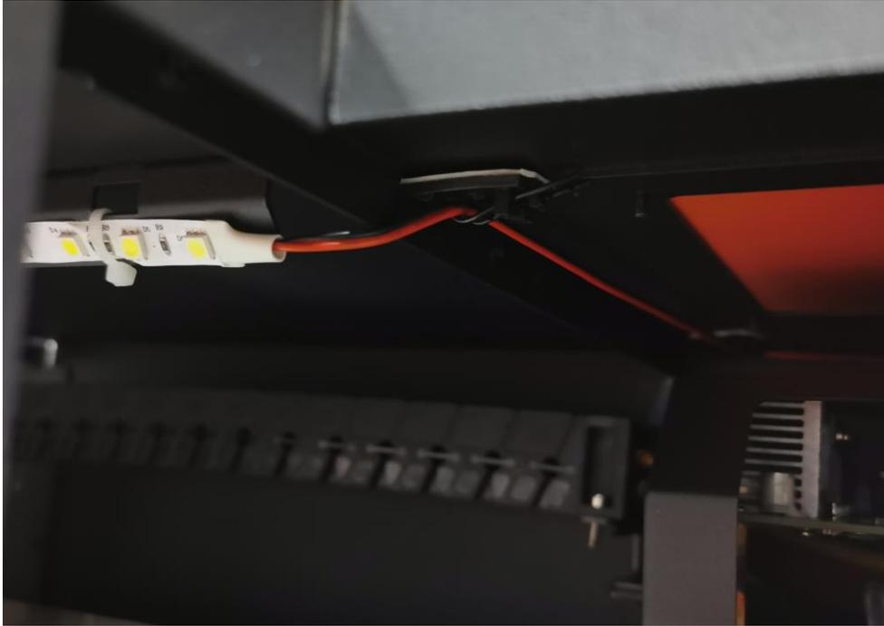
Before August 2021, the machine's LED light belt was integrated. When removing the top cover, the cable tie needs to be cut off
