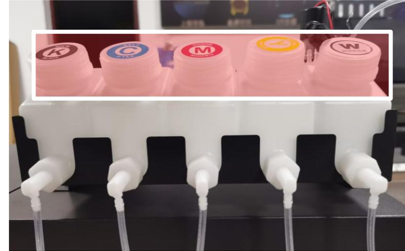
Tighten the ink cartridge cover to prevent ink leakage
