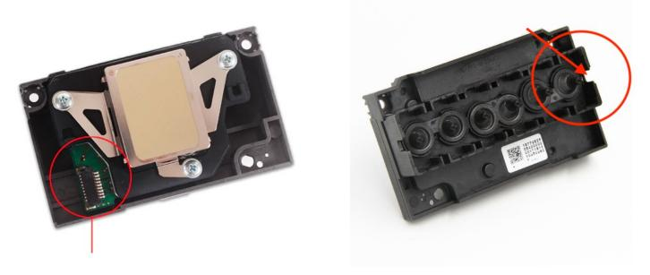
We **DO NOT recommend** you do any DIRECT or MANUAL FLUSHING, **unless** you are completely sure that you have NO serious NOZZLE CLOGS. If you intend to Flush the printhead, and you have a serious clog, you should **REMOVE the printhead from the printer first.** Then proceed to clean and flush.
