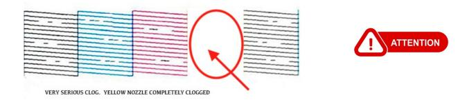
DO NOT DO ANY MORE CLEANINGS, OR FLUSHINGS while the printhead is in the printer. The printhead must be removed from the printer.
