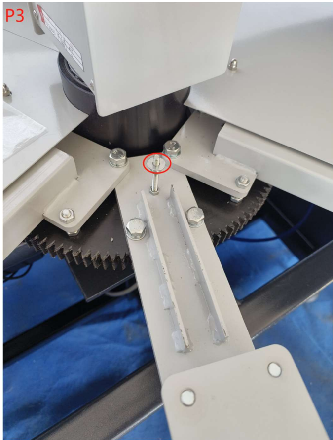
P3: Put a flat washer at the marked position.
